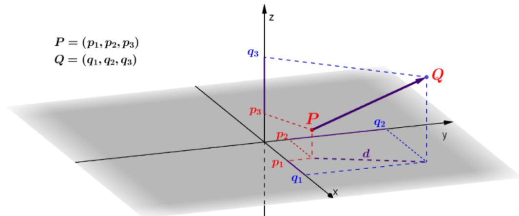
$$\left. \begin{aligned} d(P, Q) &= |\overrightarrow{PQ}| \\ d(P, Q) &= \sqrt{d^2 + (q_3 - p_3)^2} \\ d &= \sqrt{(q_1 - p_1)^2 + (q_2 - p_2)^2} \end{aligned} \right\} \Rightarrow d = \sqrt{(q_1 - p_1)^2 + (q_2 - p_2)^2 + (q_3 - p_3)^2}$$
