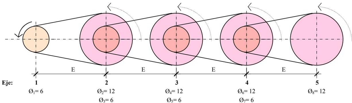
Velocidad:  $n_1 = 16$  rpm       $N_2 =$  \_\_\_\_\_ rpm       $N_3 =$  \_\_\_\_\_ rpm       $N_4 =$  \_\_\_\_\_ rpm       $N_5 =$  \_\_\_\_\_ rpm
