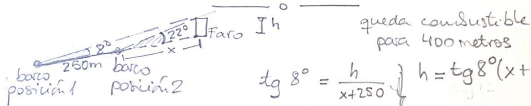
$$\begin{aligned} \operatorname{tg} 8^\circ &= \frac{h}{x+250} \\ \operatorname{tg} 22^\circ &= \frac{h}{x} \end{aligned} \quad \left. \begin{array}{l} h = \operatorname{tg} 8^\circ (x+250) \\ x = \frac{h}{\operatorname{tg} 22^\circ} \end{array} \right.$$
