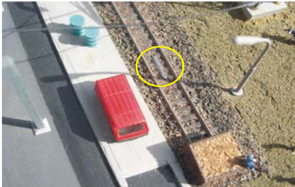
Figure 15. Reed relay placed between the rails
