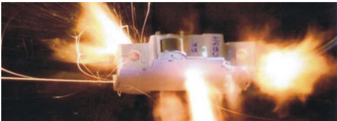
Figure 8: Sparks and noise at testing of MCBs subjected to currents of several thousand amperes
