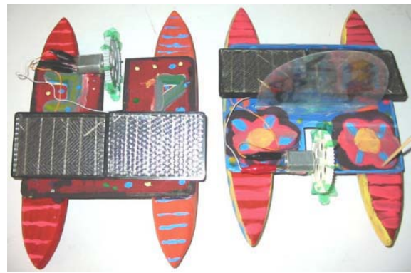
Photo 12. Two solar "river boats" with paddle-wheels made out of gears with attached plastic fins cut out of plastic bottles.
