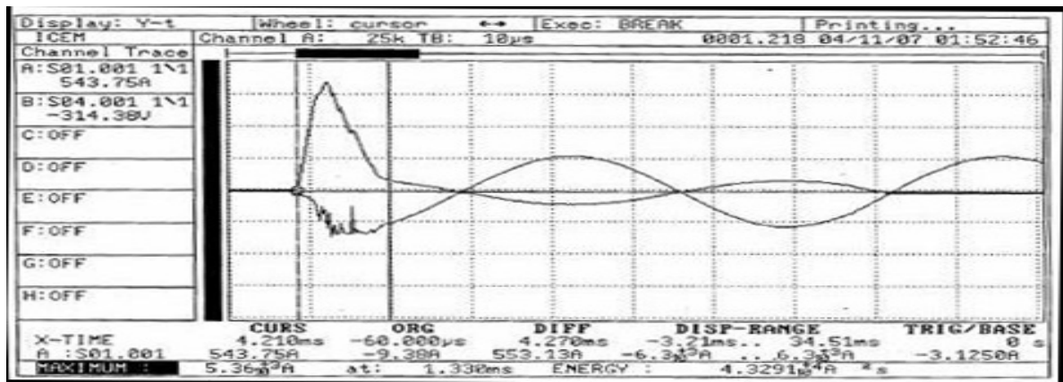
Figure 9: Current and voltage of the circuit breaker in a disconnecting (breaking) phase
