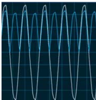
Figure 10. The registered signals from the channels of the data acquisition board in full-wave rectifier
