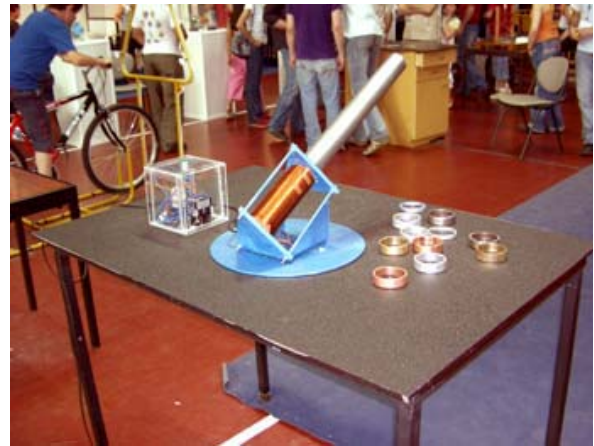
Figure 2. Ring launcher at Oficinas de Electricidade (Electricity Workshops)
