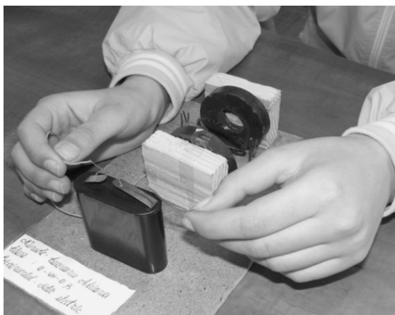
Figure 5. A simple and efficient electrical motor
