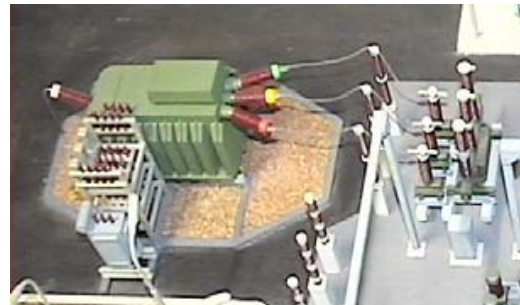
Figure 10. Close-up on main transformer (left) and circuit breakers (right)
