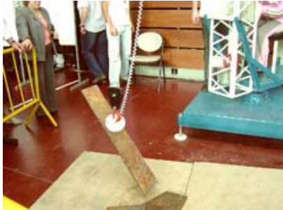
Figure 9. Electromagnet elevating an iron piece
