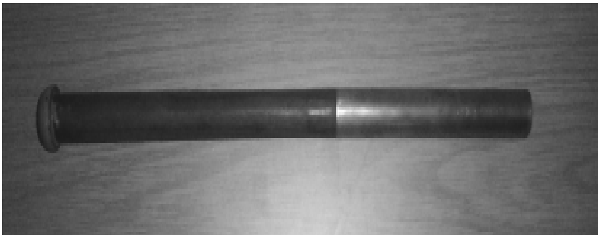
Figure 3. Two-piece rod made of iron and nylon
