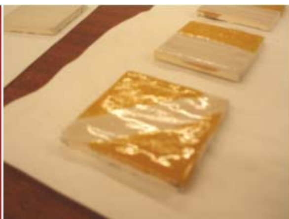
Figure 2. Azulejo produced by cold processing using polymer cross-linking
