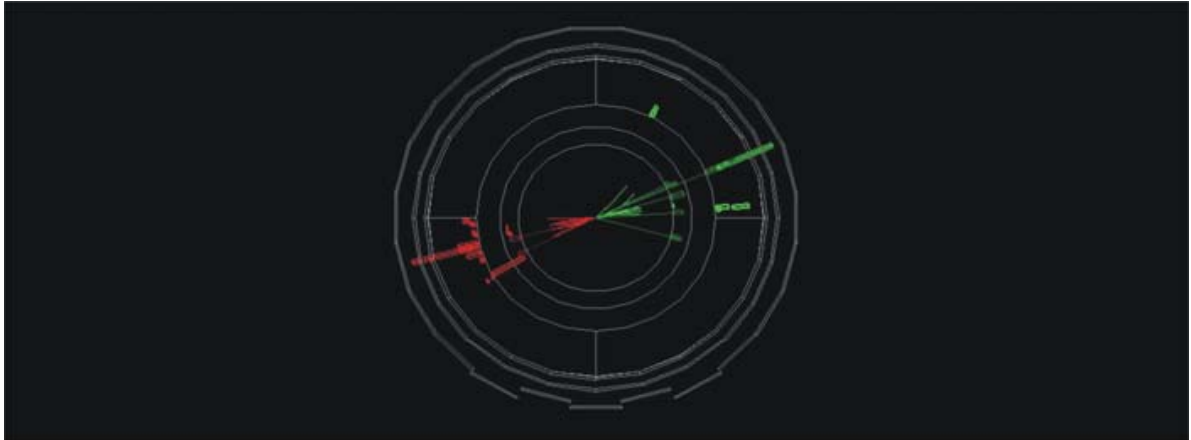
Figure 1. Two-jet event. The production of a Z^0 particle decaying into a quark and an antiquark giving rise to two jets of particles depositing their energy in the calorimeters (rectangles)
