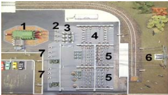
Figure 9. Electrical substation layout: 1 – main transformer with underground feeder; 2 – measurement transformers; 3 – main circuit breakers; 4 – main bus; 5 – main bus air break and disconnecting switches; 6 – outgoing main power line; 7 – outgoing secondary lines (not mounted)
