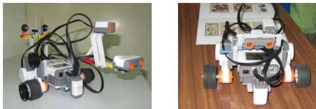
Figure 3. Two robots with the ultrasonic sensor on different locations
