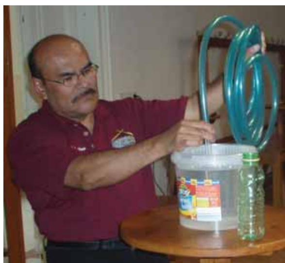
Figure 4. Single-tube apparatus to measure atmospheric pressure
