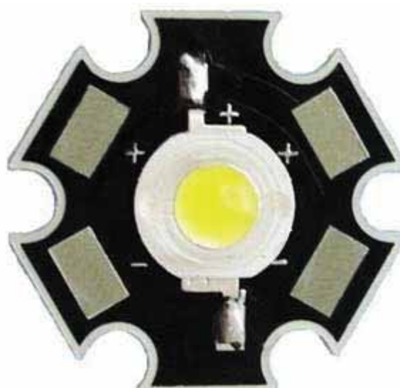
Figure 5. Power LED mounted on the star aluminum
