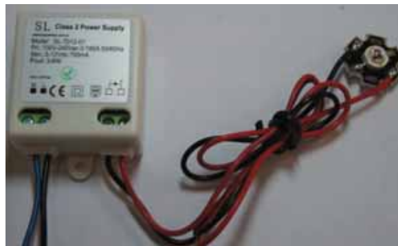
Figure 4. 6 watt commercial power source and power LED
