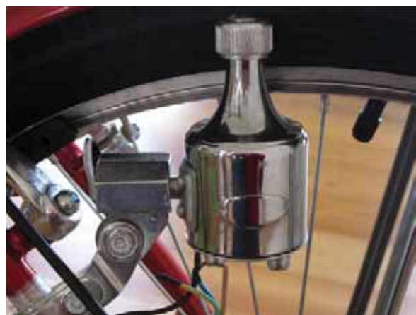
Figure 4. AC voltage generator fitted in the back wheel frame of a bicycle
