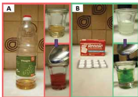
Figure 3. Students could use red cabbage extract to check the pH of the following substance: (A) vinegar and (B) and antacid tablet (bicarbonate). At the top-right corner of each picture there is a glass filled with one of the three tested substances and at the bottom-right corner these substances after adding some drops of red cabbage extract
