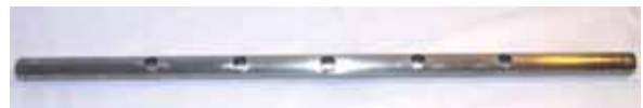
Figure 5. One of the upper horizontal pipes of the bearing structure. The tips of the nylon wires holding the snooker balls pass through the holes in the pipe and then are tied to it. The distance between the holes is the diameter of the snooker balls
