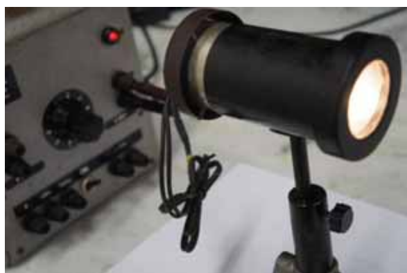
Figure 6. Optical Source of Leybold Optics using incandescent lamp
