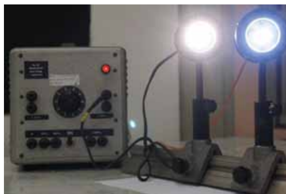
Figure 9. Final appearance of the light source assembly. Aside the power supply is the incandescent lamp assembly and at right that with power LED connected directly to mains
