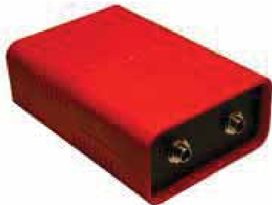
Figure 5. Box containing a rectifier, a filter and a voltage limiter for each lane
