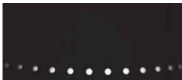
Figure 13. Photograph obtained from a simple pendulum highlighted under motion with a strobe LED
