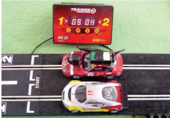
Figure 6. Two slot cars on the track, near a lap counter. A wireless camera, powered by a 9V battery is attached to the car running on lane 2, closer to the lap counter
