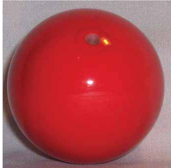
Figure 3. Snooker ball with a drilled hole. A brass wire holder will be fastened to the ball with a steel screw
