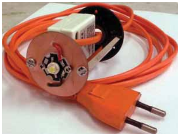
Figure 8. Installation of a LED with a commercial constant current source
