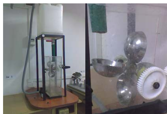
Figure 7. Water energy: a model of a pumped-storage hydroelectric power station. The turbine is made of ladles
