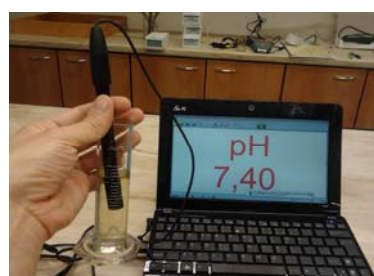
Figure 4. Measuring pH of a soil suspension in water using Vernier sensor.
