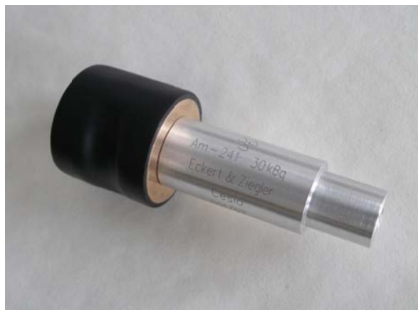
Figure 1. School gamma radiation source SZZ Gama 30 kBq
