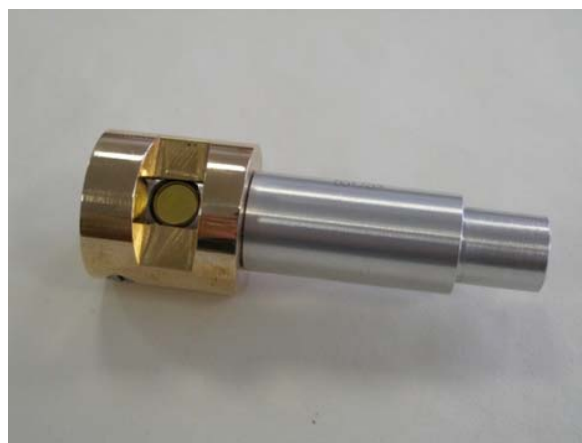
Figure 2. Emitter of SZZ Gamma 30 kBq
