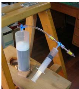
Figure 2a. The hanging type with an air pump
