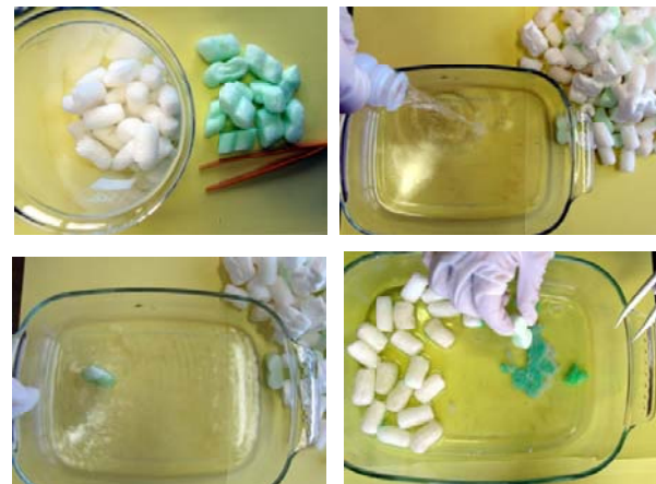
Figure 7. Example for illustrating the different chemical reactivity depending on the structure. The polypropylene foam (white) dissolves slower than the polystyrene foam (green) in acetone [17].
