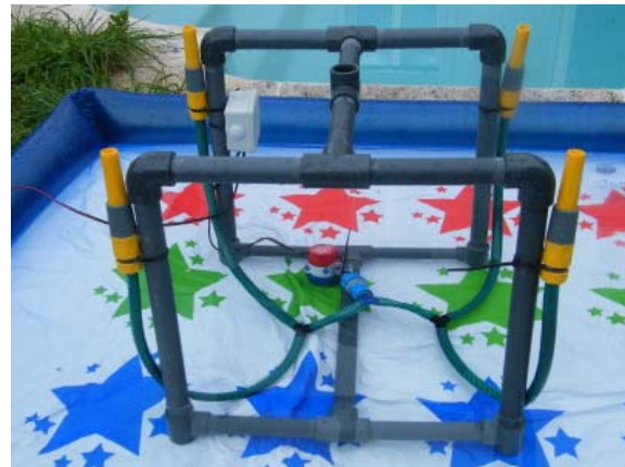
Figure 6. Structure with pump and hoses
