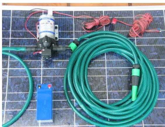
Figure 4. The solar pumping set
