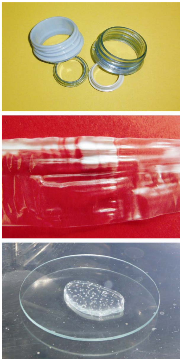
Figure 3. Thread of PET before (transparent) and after the introduction into boiling water (up). Opacity generated in PP when it is stretched (centre). HDPE transparent obtained when it is heated above 140°C (down).
