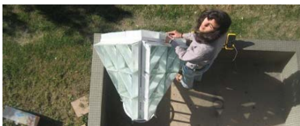
Figure 17.A. Triangular pyramid Skylight test
