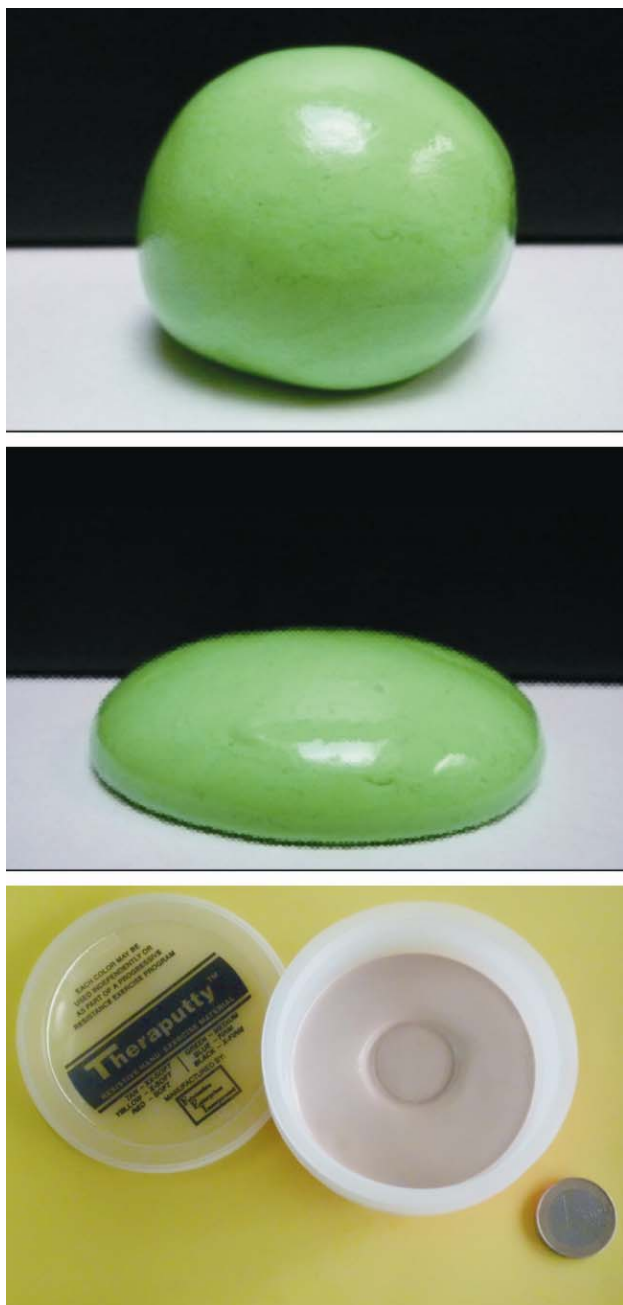
Figure 5. Illustration of the viscous behaviour of the Silly Putty®: ball (up) that is spilled on a flat surface (centre) and disappearance of the bas-relief of a coin with time (down).
