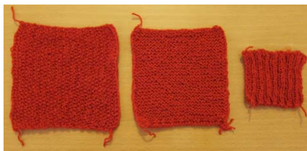
Figure 1. (left) Rice pattern: 4,4 lines/cm and 2,5 stitches/cm; (middle) knit stitches: 5,5 lines/cm and 2,7 stitches/cm; (right) 2 knits 2purls: 3,53 lines/cm and 3,57 stitches/cm.
