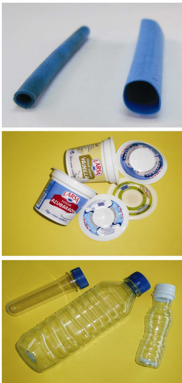
Figure 6. Shrink PE before and after submitting to heat source (up). Recovering of the original shape (a sheet) of yogurt glass made with PS (centre). Tendency to recover the original shape (cylinders or perform) of PET bottles (down).
