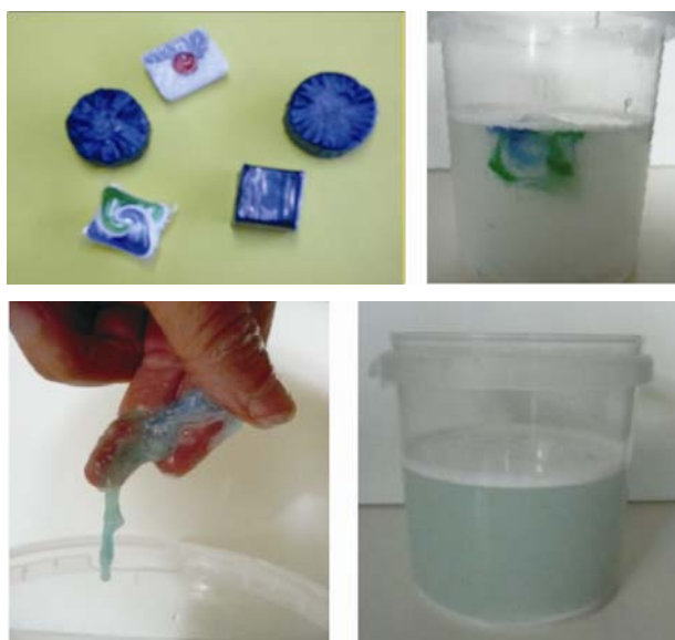
Figure 7. Different type of commercial products covered with plastics soluble in water (up-left) and illustration of the plastic dissolution when the tablet is immersed in warm water.
