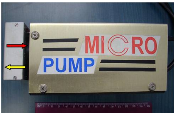
Figure 3. ISES Digital burette (The inlet (red arrow) and outlet (yellow arrow) of the liquid are denoted)
