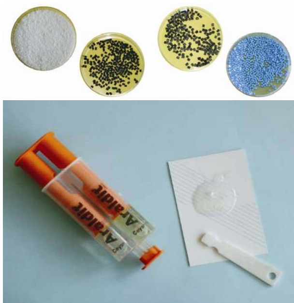
Figure 1. Examples of different types of thermoplastics under pellets shape (up) and a commercial thermosetting (Araldit®) made by two precursors (down).
