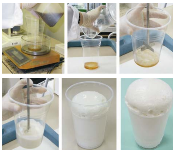
Figure 8. Different stages of the manufacturing process of a foam.
