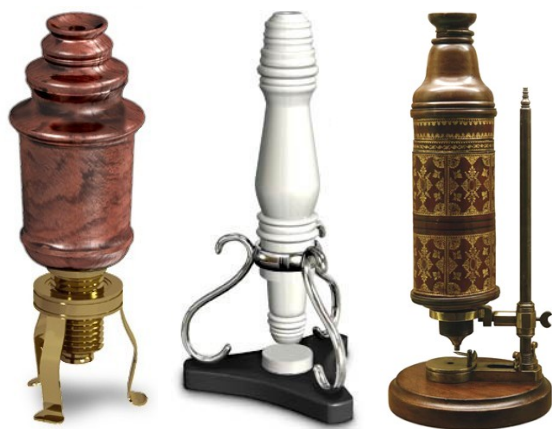
Figure 2: Divini's vase-shaped microscope (left), Campani's ivory turned monocular microscope (centre) & Cock's compound microscope, manufactured in London for R. Hooke (right).
