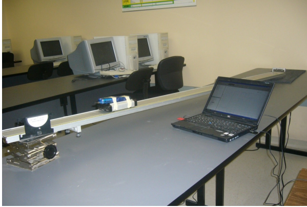
Figure 1. Experimental setup of the 3-axis accelerometer - altimeter mounted on cart on inclined ramp.
