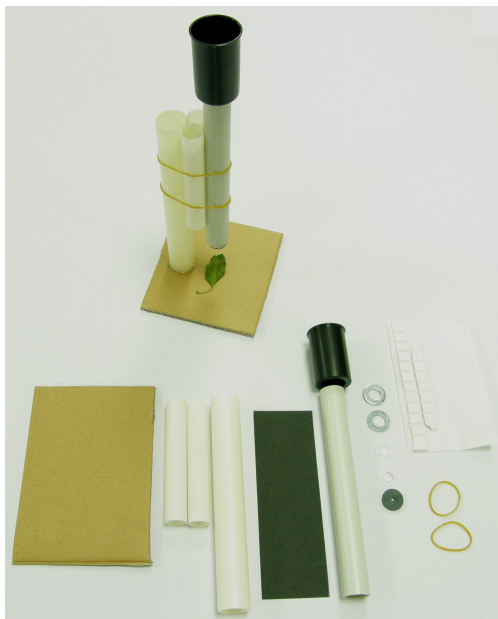
Figure 6: The materials used & the first version of the constructed microscope with 2 lenses.
