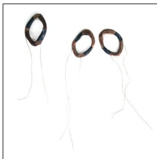
Figure 1 – Constructing the coils for the first device
