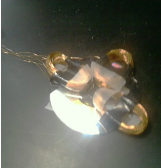
Figure 2 – Building the stator
