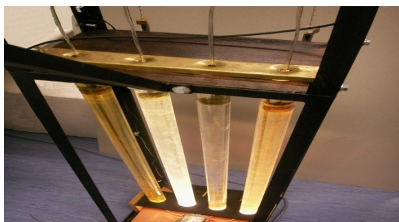
Figure 5. Apparatus of the hydrostatic law experiment
