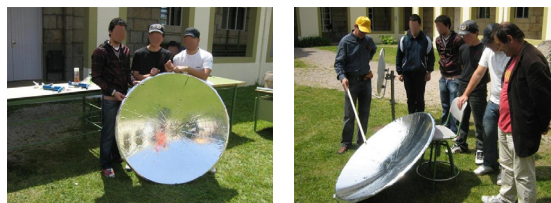
Figure 20. Finishing and testing reflector
