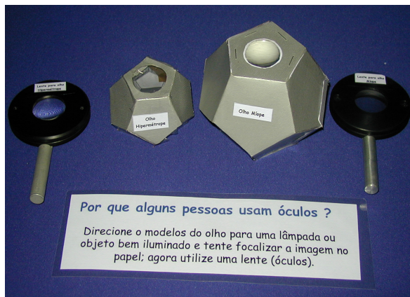
Figure 6 – Dodecagon manufacture for the myopia and hyperopia models with their respective corrective lens simulating the glasses that the people must carry. At the bottom is an instructive text in Portuguese to operate the experiment.
