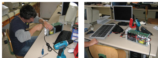
Figure 16. Electrification kit with solar recharged UPS
