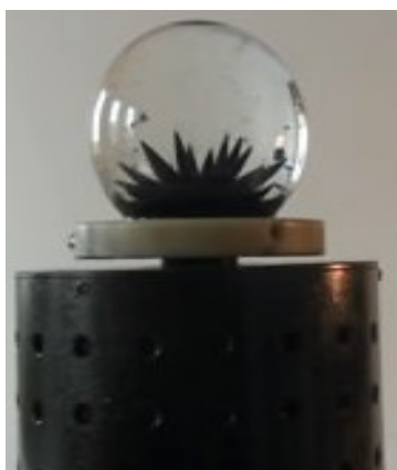
Fig. 4. The magnetic field of electromagnet showed by ferrofluid.
