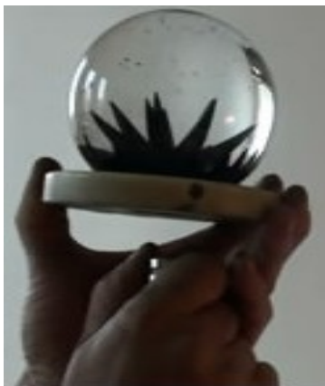
Fig. 3. The magnetic field of permanent magnet showed by ferrofluid.
