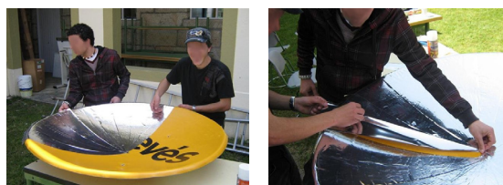
Figure 19. Applying reflective sheet
