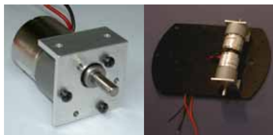
Figure 11. L shape Motor support (left) and robot base with two motors on (right)
