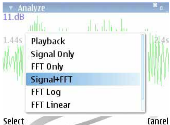
Figure 5. Analysis options that can be applied to the signal section selected includes sound Playback and multiple display views of results
