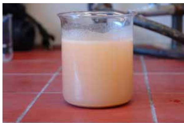
Figure 2. Waste water before clarification
