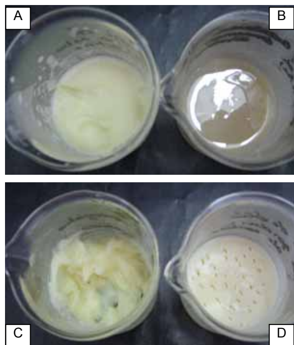
Figure 4. Soap made from several kinds of fat. A) ox tallow; B) soy oil; C) chicken fat and D) ox rib fat
