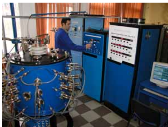
Figure 4. Industrial Unit for Tungsten thin films deposition by "Combined Magnetron Sputtering and Ion Implantation"( CMSII) technology
