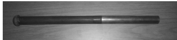
Figure 3. Two-piece rod made of iron and nylon
