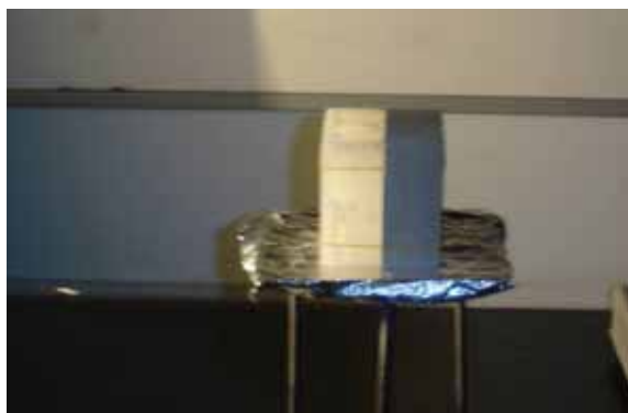
Activity 2. Verification of inverse square law – Simple photometer construction.
