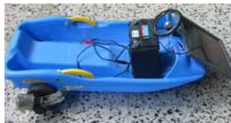
Photo 12: A “big toy car” with a PV cell and a battery, which can carry a child (Escola Antré Soares, Braga, PT with Maria da Graça Martins Pereira de Moura, Esperança Fernandes, Avelino Garrido and collaborating teachers)
