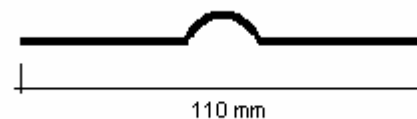
Figure 5. Side view of the iron bars used to make the traverse bar of the rotor core
