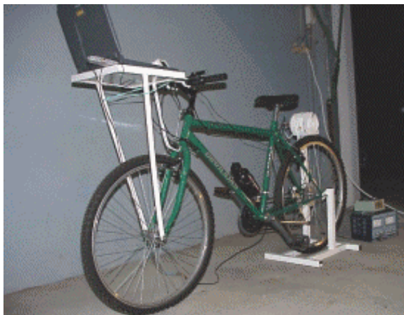
Figure 1. The homemade cycle-ergometer
