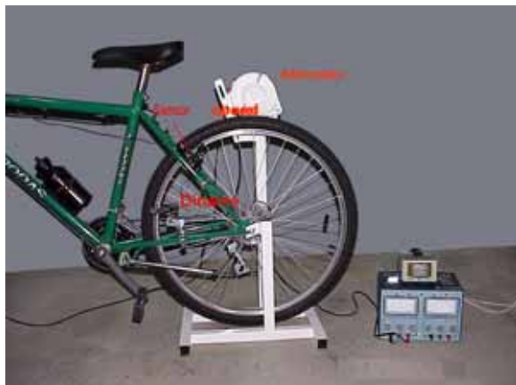
Figure 2. Details of the coupling of the electromagnetic energy conversion units to the stand-still bicycle
