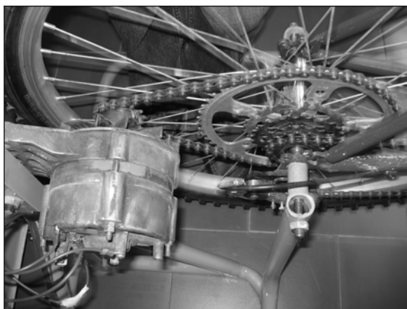
Figure 3. Car alternator linked to the rear wheel of the bicycle
