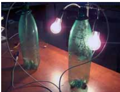
Experimental set-up for studying the effect of the CO 2 emissions on the atmosphere
