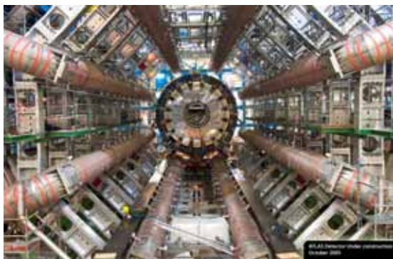
Figure 4 The ATLAS detector under construction at CERN. The man at the bottom of the photo indicates the scale of the detector
