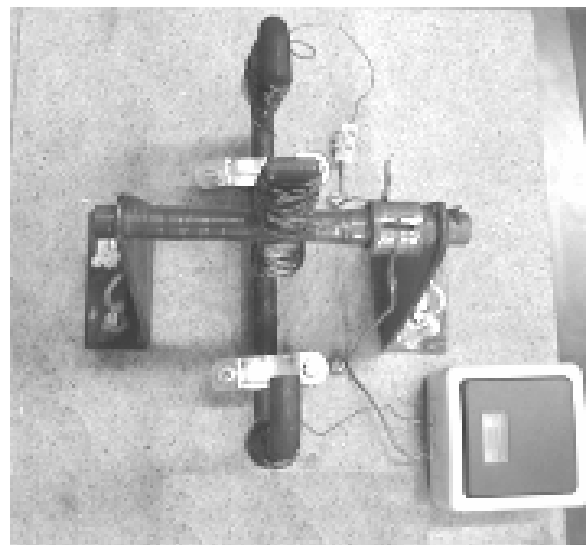
Figure 1. Handmade universal series motor
