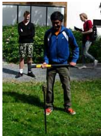
Fig. 3 Preparing the measurement of Radon under ground
