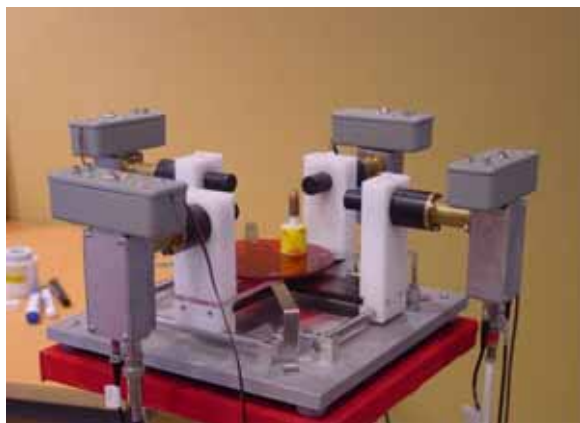
Fig. 2 A simple PET camera. Each pair of movable detectors is coupled in coincidence. During the demonstrations the source is covered
