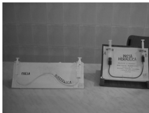
Figure 2. Experimental devices: hydraulic pumps
