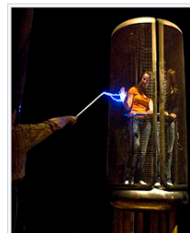
Faraday cage demonstration on volunteers in the Palais de la Découverte in Paris
