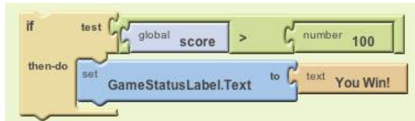
Figure 16-8. Using the global score block to get the value stored in the variable
