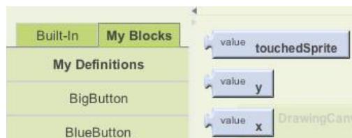
Figure 2-8. The system has added references to the event arguments touchedSprite , y , and x
