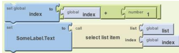
Figure 19-7. Incrementing the index value and using the incremented value to select the next list item
