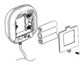
4. Refit the battery cover by fastening its screw.
