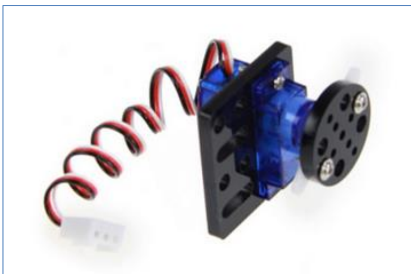
Micro Servo 9g (servomotor)
