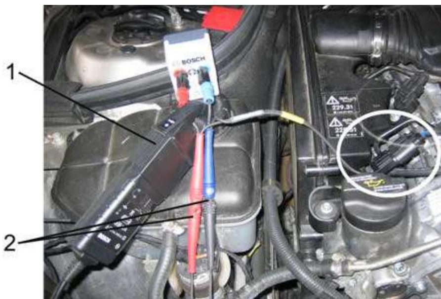
1 = Current measurement (current probe)
