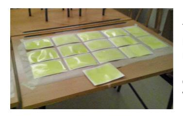
These are paper sheets that have been **coated** with a material which is sensitive to UV light (sunlight). The kind of paper must be resistant to water.
