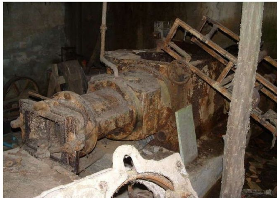
MÁQUINA "GALLETERA" QUE FABRICABA AS TELLAS E LADRILLOS
